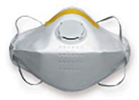
This mask has a polypropylene outer, inner and support layer, a natural rubber elastic band and a polyethylene-coated wire nose part. Protects from non-toxic solid and liquid aerosols, calcium carbonate, kaolin, cement, cellulose, sulphur, cotton, flour, coal, ferritic steel, vegetable oils and soft wood. It is specifically indicated for the textile industry, crafting, metallurgy, mining, underground public works, carpentry and woodwork.
